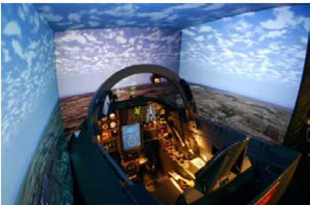
Randolph Air Force Base, Texas. The T-38C Talon trainer's "glass cockpit" features the digital instrument displays in aircraft and virtual reality views of realistic flight environments. (U.S. Air Force photo by Javier Garcia)
